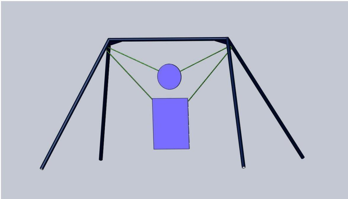
The metal plates for shooting distances up to 300 meters should be made from steel sheets with 16-20 mm thickness, in order for them to be relatively heavy enough, so that they don't roll or turn over, after a hit.
